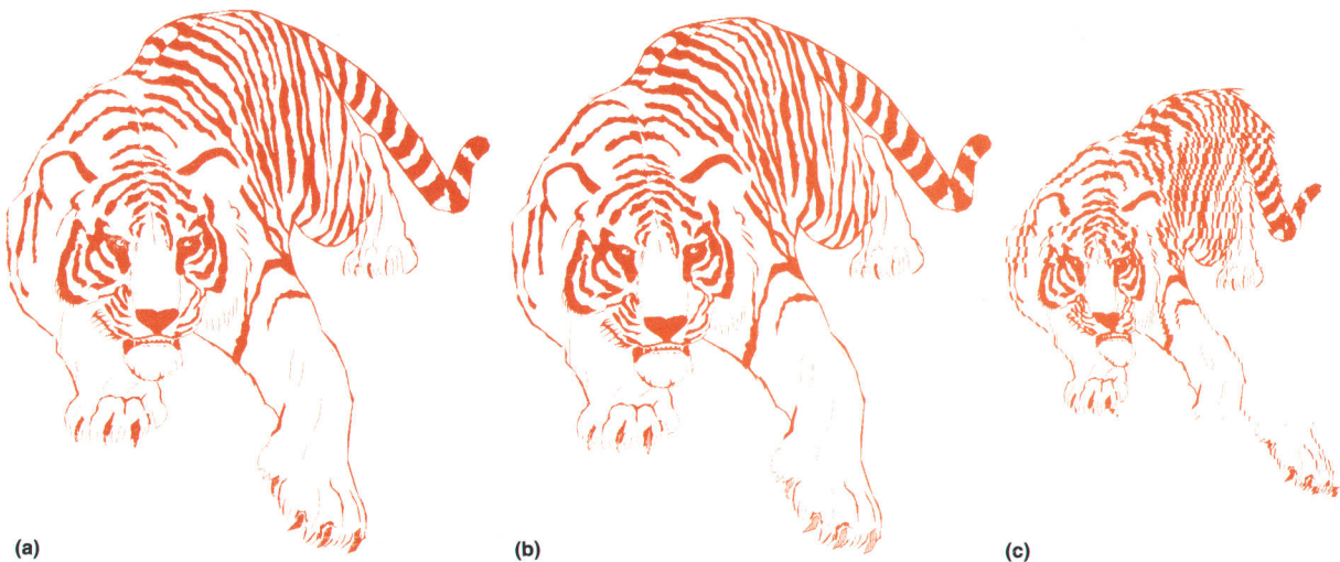
Fig. 2. (a) Epson FX-80 printer output. (b) Output of HP DeskJet printer with Epson FX-80 emulation cartridge for same input. (c) Output of another printer without scaling ability.
