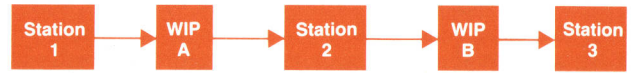
Fig. 6. Simplified diagram of the HEDS-9000 production line, showing work-in-progress (WIP) holding areas and workstations. The line operates under a pull system.
